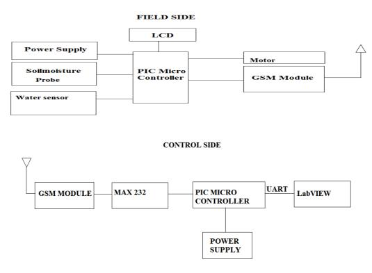
Figure 1.Block Diagram Of Wireless Monitoring And Controlling Automatic Irrigation Field
